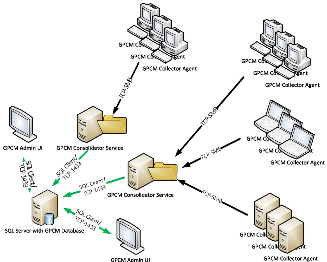
Figure 4 A typical large-scale GPCM deployment.
